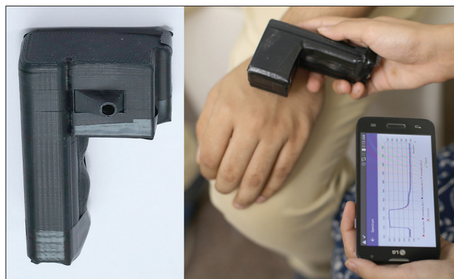
Figure 2: Use of fluorescence spectrometer in capturing fluorescence spectra and transfer via Bluetooth to mobile phone
