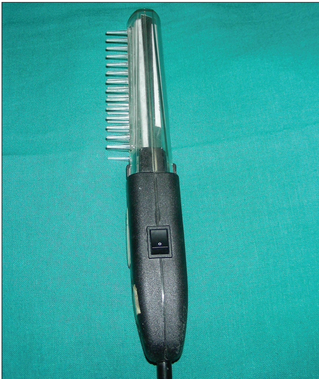
Figure 1: Hand-held narrow band ultraviolet B comb (V-Care Meditech Pvt. Ltd., Bengaluru, India)
