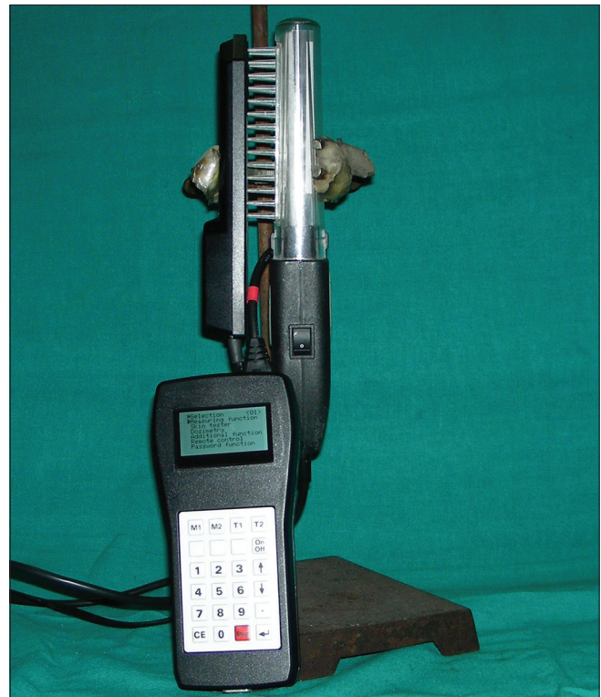
Figure 2: Calibration of irradiance of narrow band ultraviolet B comb using an integrated ultraviolet meter (Herbert Waldmann GmbH and Co. KG Villingen-Schwenningen, Germany)
