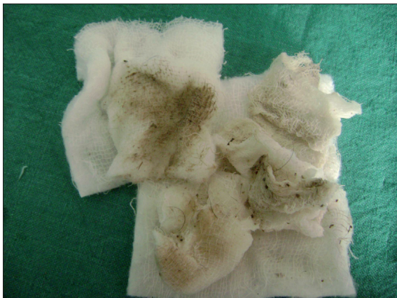
Figure 2: Alcohol swab test showing dirt and debris
