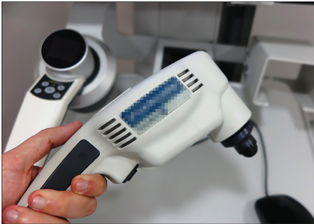
Figure 1b: The handheld device simplifies examining difficult to access skin regions such as the interdigital folds and allows the modification of the cutaneous depth examination, through a button system placed on the device itself
