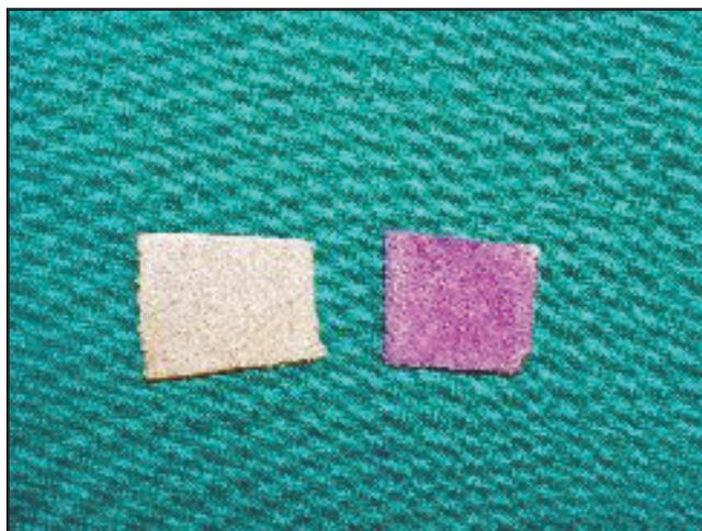
Figure 1: Untested leather and leather testing positive to chromium by diphenyl carbazide (DPC) spot test
