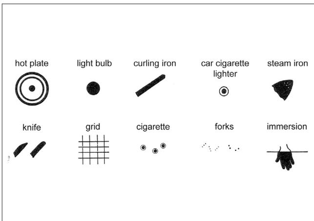
Figure 5: Burn marks of heated objects<sup>[4]</sup>
