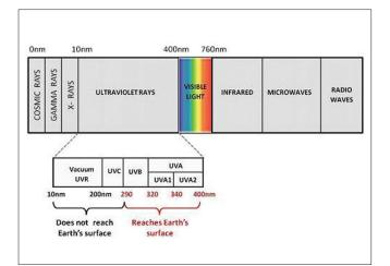
Figure 1: Electromagnetic spectrum of sun
