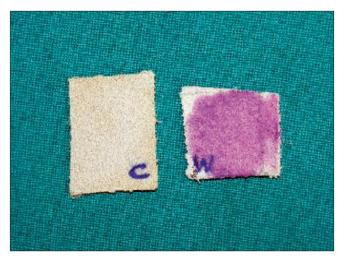
Figure 2: DPC spot test: negative in vitamin C-treated leather and positive in leather soaked in distilled water
