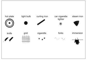
Figure 5: Burn marks of heated objects<sup>[4]</sup>
