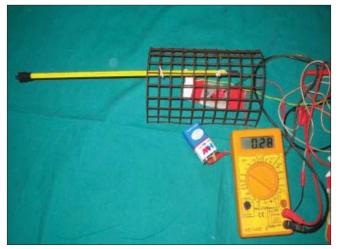
Figure 1: Open hood with heater and thermometer
