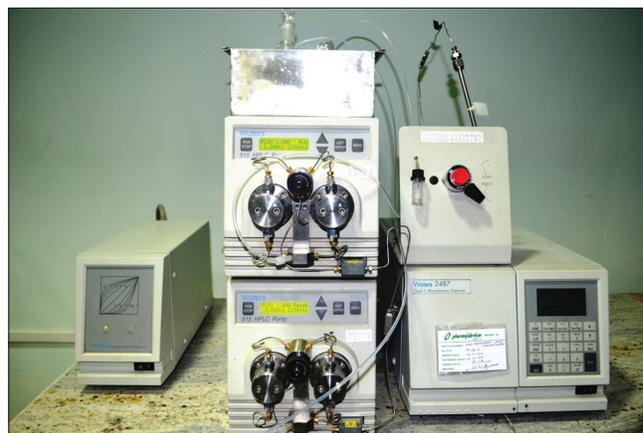
**Figure 2: High performance liquid chromatography-equipment**
