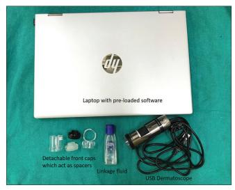
Figure 2: A universal serial bus dermatoscope with accompanying requirements for capturing and storing images
