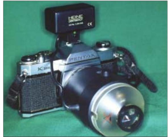
**Figure 4:** Dermaphot, a dermoscope with image capturing capability.
