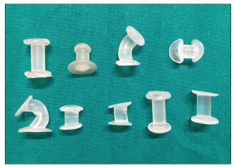
Figure 3: Different molds prepared from a glue stick
