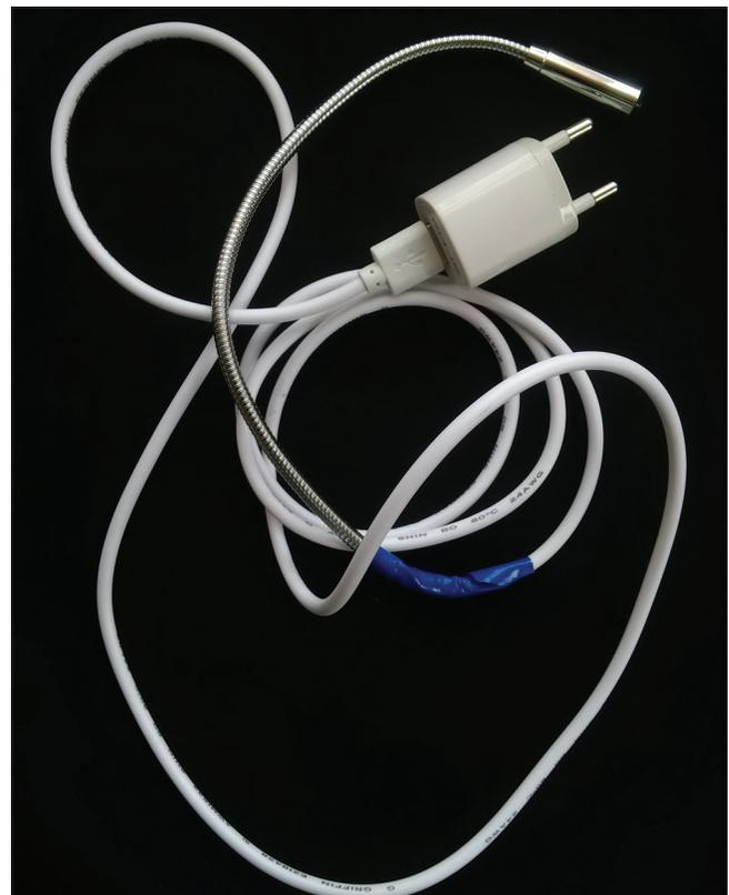
**Figure 2a:** The light source with a mobile phone charger as the power source
