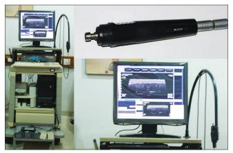
Figure 1b: Ultrasound biomicroscopy machine with 35 and 50 MHz probes
