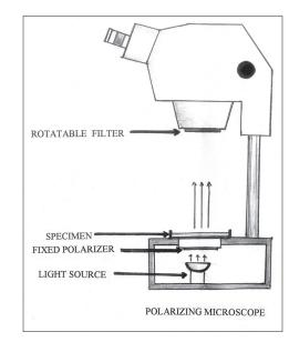
Figure 1: Principle of polarizing microscopy
