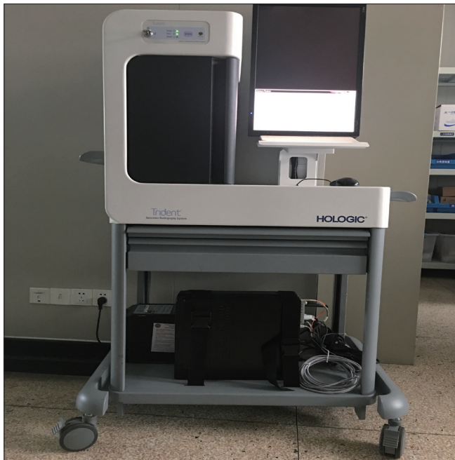
Figure 1: View of the specimen radiography system (HOLOGIC, Marlborough, MA, USA). This mobile digital specimen radiography unit is composed of a display device, computer and screening box. The system can be easily moved into the operation room.
