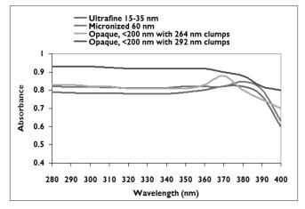
Figure 1: Absorbance spectra for zinc oxide particles of varying sizes<sup>[10]</sup>
