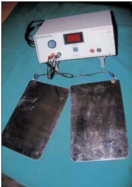
**Figure 1:** Iontophoresis machine
