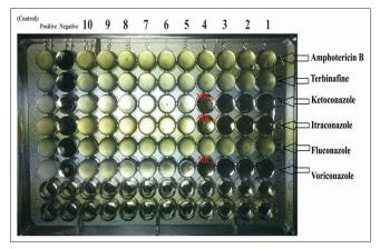
Figure 4: Minimal inhibitory concentrations by microdilution method in round-bottomed 96-well microdilution tray
