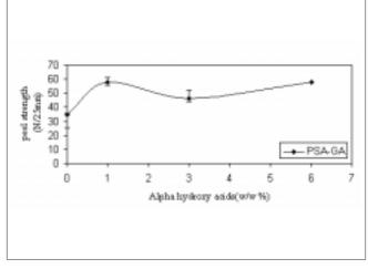
Figure 2: A plot of peel force versus GA concentration for 30 µm adhesive layer thickness (n=3)
