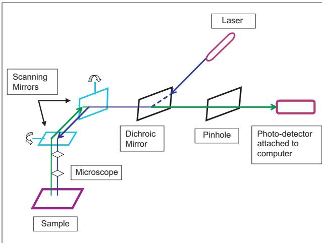
**Figure 2: Diagrammatic representation of principle of confocal microscopy**
