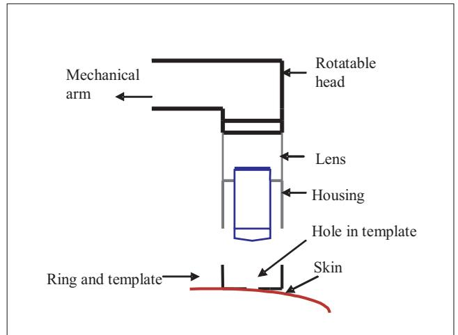
**Figure 3: Line diagram showing the structure of skin contact device of confocal laser microscope**
