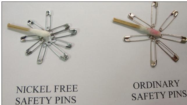
**Figure 1: Dimethyl glyoxime spot test to demonstrate the absence of nickel**
