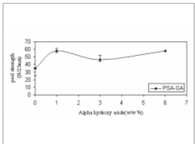
Figure 2: A plot of peel force versus GA concentration for 30 μm adhesive layer thickness (n=3)
