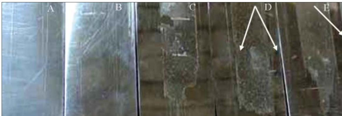
**Figure 3:** Peel test plates of PSA containing 3 and 6 (w/w %) of GA (A and B respectively) and 1, 3 and 6 (w/w %) of LA (C, D and E respectively)
