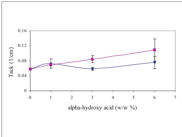
**Figure 4:** A plot of Tack versus concentration of (♦) GA and (■) LA for 30 µm adhesive layer thickness (3) (n=3)
