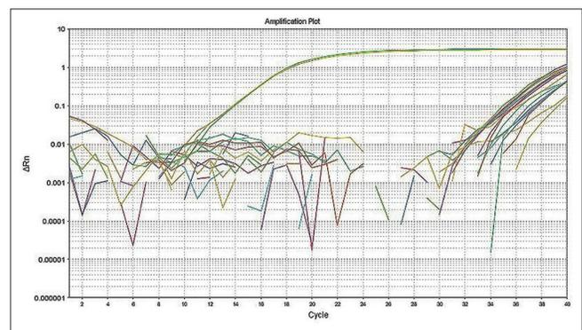
**Figure 2b:** Specificity of quantitative polymerase chain reaction primers for detection of *M. leprae* was tested using DNA from other organisms.
