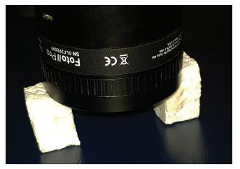
Figure 4: Spacer attached to Dermlite Foto ii pro
